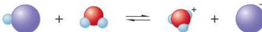
FIGURE 14.2 The reaction of an acid HA with water to form \text{H}_3\text{O}^+ and a conjugate base \text{A}^- .
