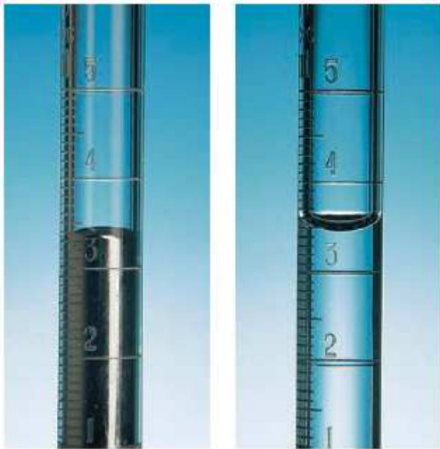
FIGURE 10.7 Nonpolar liquid mercury forms a convex meniscus in a glass tube, whereas polar water forms a concave meniscus.
